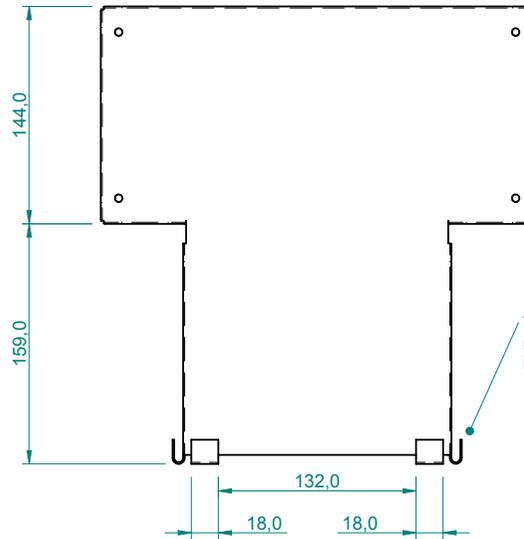
Tabs (4 of) to be formed around the wire mesh back panel to secure the feeder platform in position.
