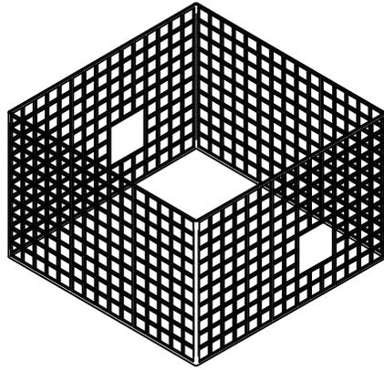
Open corner to be joined using cable ties or tying wire
