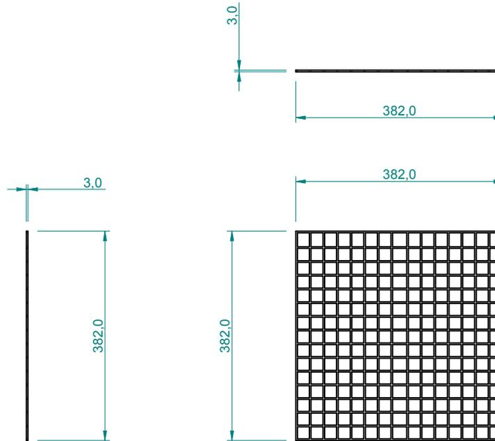
**Base to be attached to body with cable ties or tying wire**
