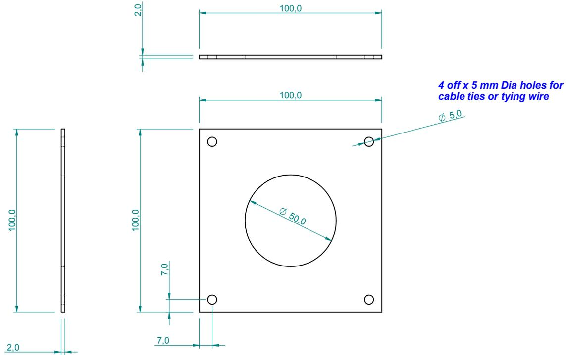
4 off x 5 mm Dia holes for cable ties or tying wire
