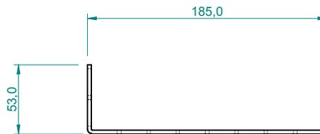
**Base to be attached to body with cable ties or tying wire**
